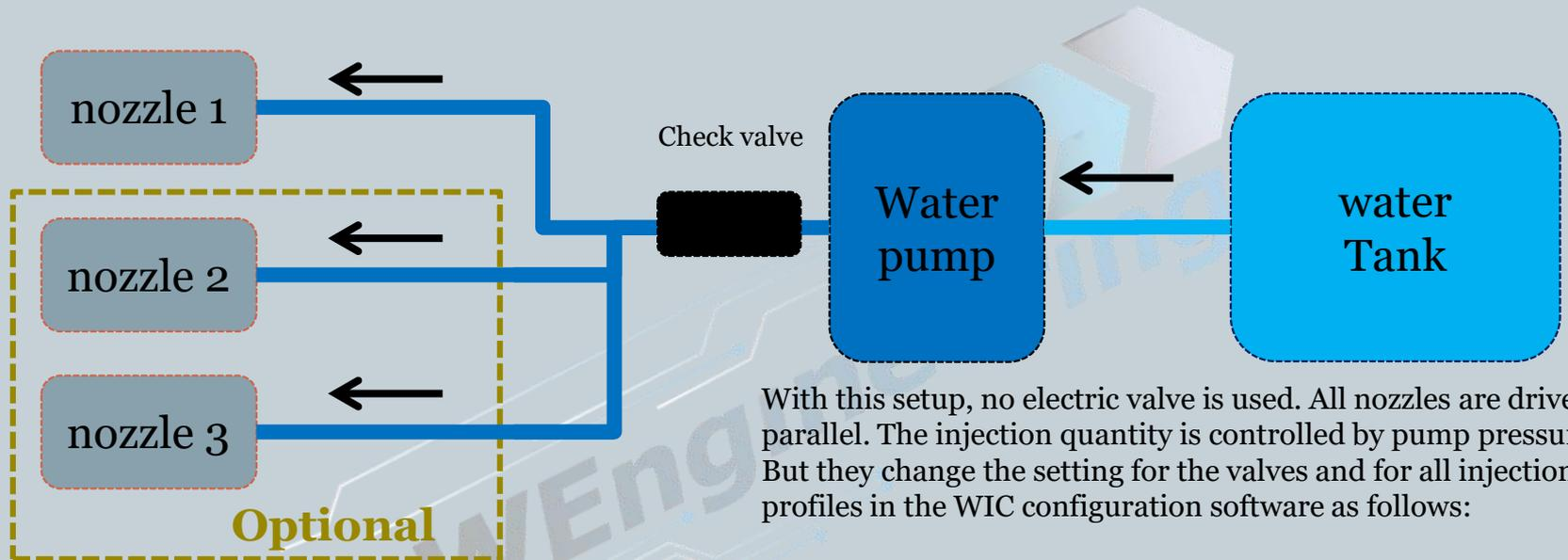
With this setup, no electric valve is used. All nozzles are driven in parallel. The injection quantity is controlled by pump pressure. But they change the setting for the valves and for all injection profiles in the WIC configuration software as follows:
