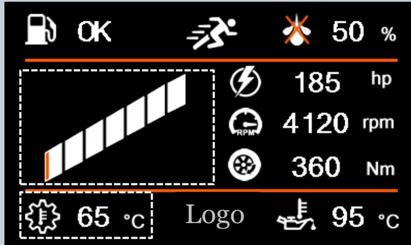
For vehicles with no gearbox temperature sensor in this area, the cooling water temperature is displayed
