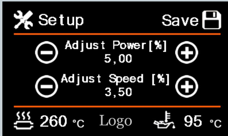
In this setup menu it is possible to correct the displayed power and speed.
