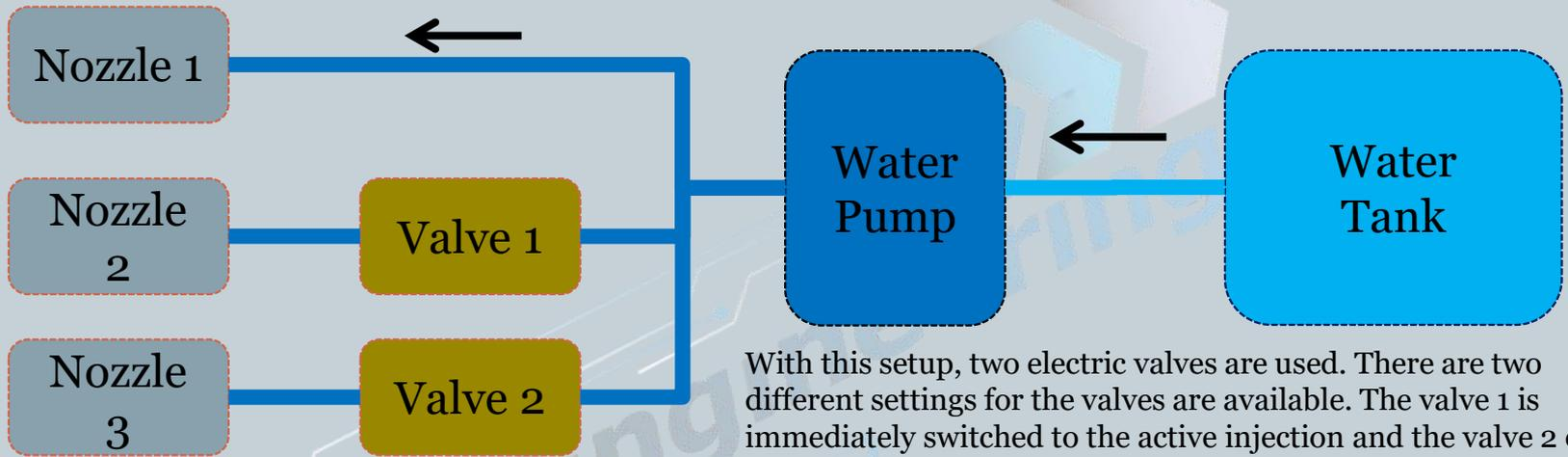
With this setup, two electric valves are used. There are two different settings for the valves are available. The valve 1 is immediately switched to the active injection and the valve 2 only from a speed of 3000U / min. The injection quantity is controlled by pump pressure. But they change the setting for the valves in the WIC configuration software as follows:
