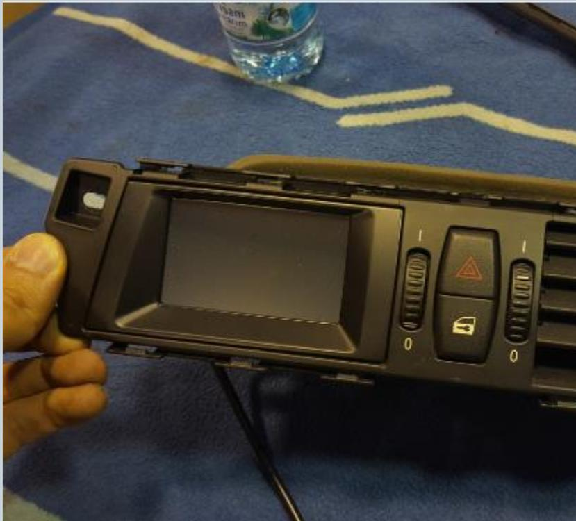
Reinstall the front part of the ventilation. The bottom side first. Now the ventilation unit can be bolted to the interior trim again.
