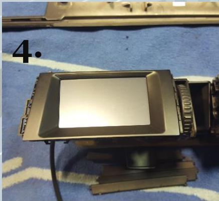
1. Unlock locks to separate the front of the vent from the rear.
