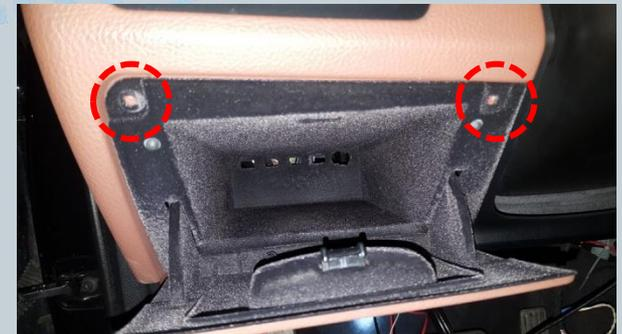
Loosen 2 screws on the storage compartment and pull out the compartment. The WIC control unit is located in this area.
