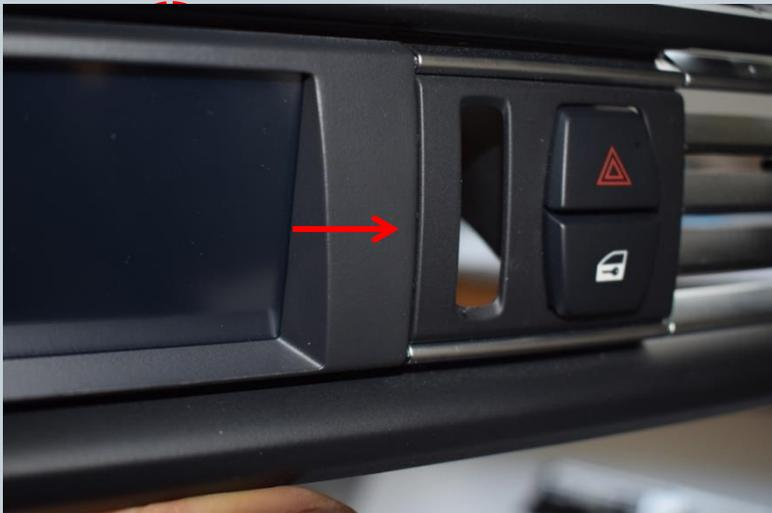
Now the left side can be snapped into place carefully. Apply a little super glue to the areas marked in red.
