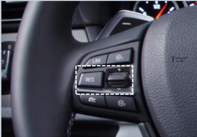
If an exhaust flap has been installed at the factory, this can be controlled using the "Res" button
