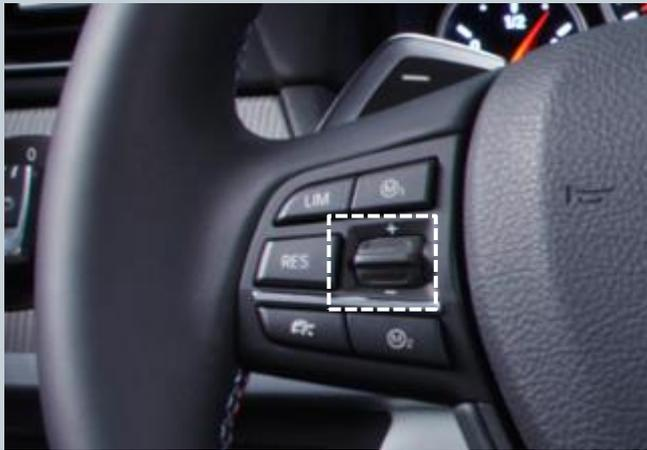
1. With the help of the wiper button on the MFL, you can quickly switch between the individual screens. To do this, press the wiper slightly up or down.
