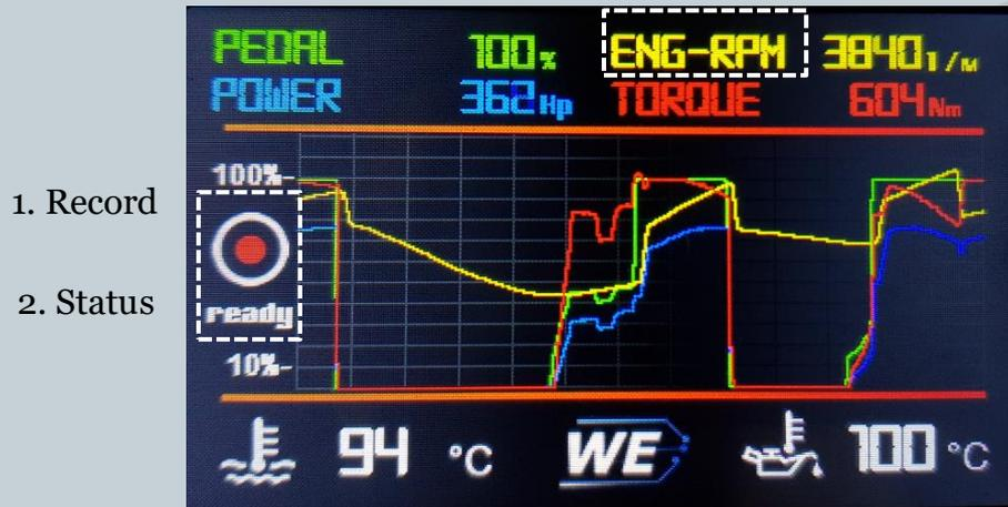
4 values can be configured as required in the graph. To do this, press the name of the signal. In the further menu you can set the signal and the scaling.
