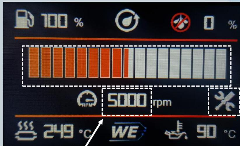
Set limit rpm for each gear number
