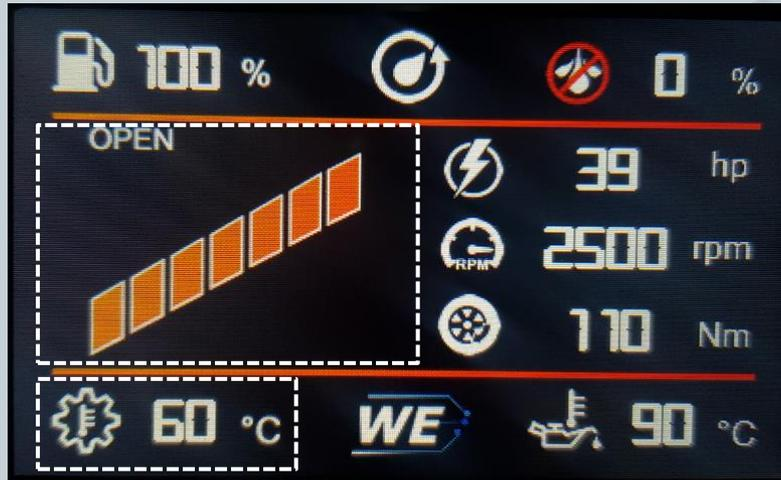
For vehicles without automatic/DCT transmission, the coolant temperature is displayed in this area. Change in setup possible.
