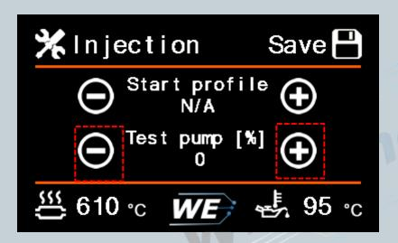
In this menu it is possible to check the functionality of the system and to make sure that the connection of the pump and the valves (if installed) was done correctly.
