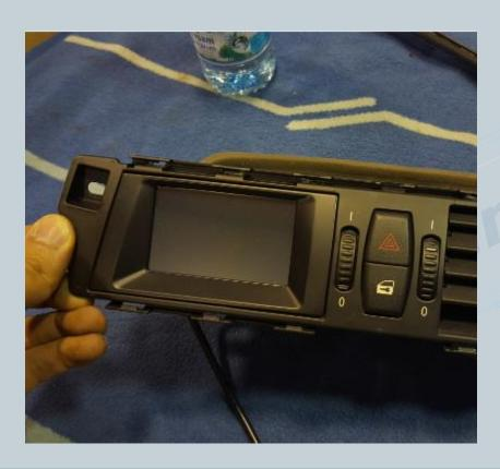
Reinstall the front part of the ventilation. The bottom side first. Now the ventilation unit can be bolted to the interior trim again.
