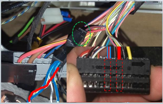
Connect the supplied CAN cable as shown in the picture (Highlighted in red).
