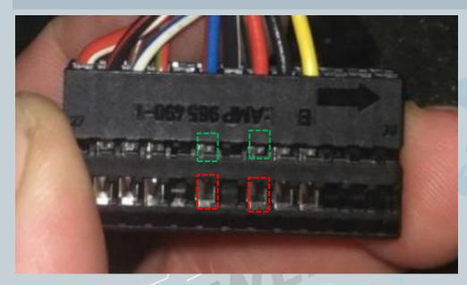
Disconnect the CAN cable (blue / red and red is twisted).
