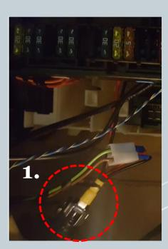
1. The supply for the control unit can be taken from the 12V charging socket.
