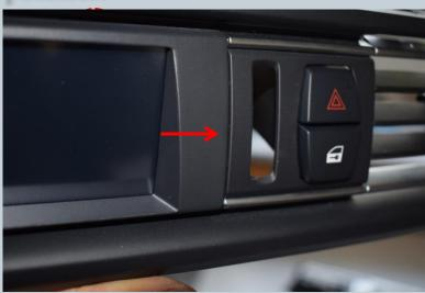
Now the left side can be snapped into place carefully. Make sure that no mandrel is broken off for attachment.
