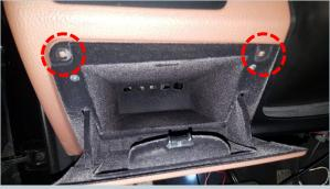
Loosen 2 screws on the storage compartment and pull out the compartment. The WMI control unit is located in this area.
