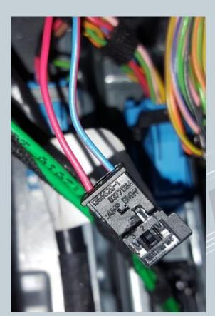
Pin the spun CAN cable into the connector supplied. Thereby "blue / red" on pin\_1 and "red" on pin\_3. The numbering is marked on the connector.
