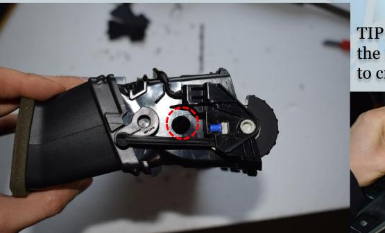
TIP: Secure the cable from the inside using cable ties to create a strain relief.
