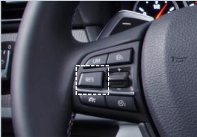
If an exhaust flap was installed at the factory, it can be controlled by pressing the "Res" button. There are 3 modes (Auto, On and Off).
