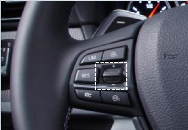
The rocker switches on the MFL can be used to switch quickly between the individual screens. To do this, push the rocker switch slightly upwards or downwards.
