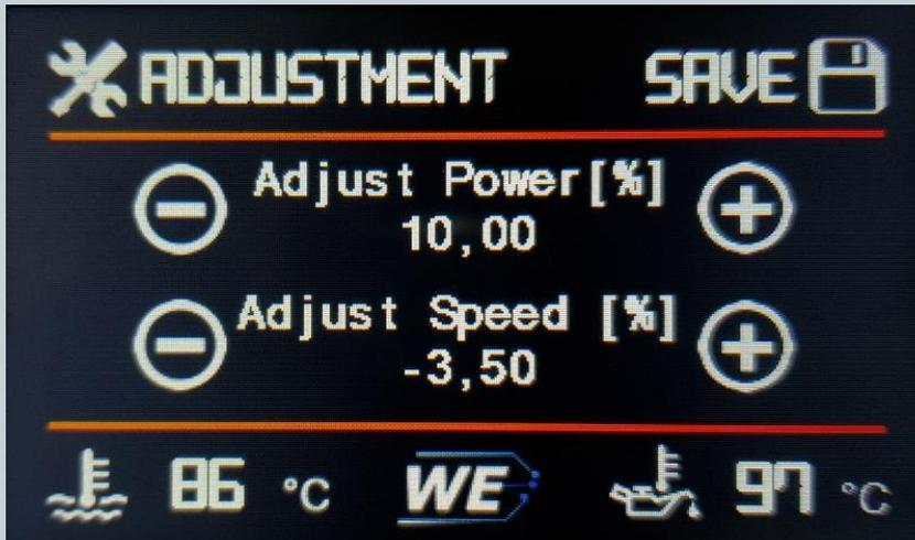
In this setup menu it is possible to correct the displayed power and speed.
