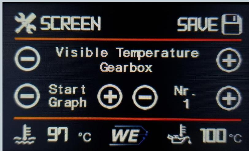
**Visible Temperature:** Whether the gearbox temperature or water temperature should be displayed in the Dash. (Only with automatic)
