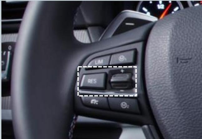
By pressing the rockers for 2 seconds, a function can be triggered in **the corresponding menu.**
