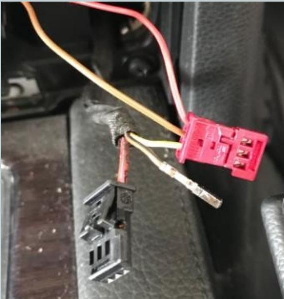
1. Open the lock on the 3-pole SZM Plug.
