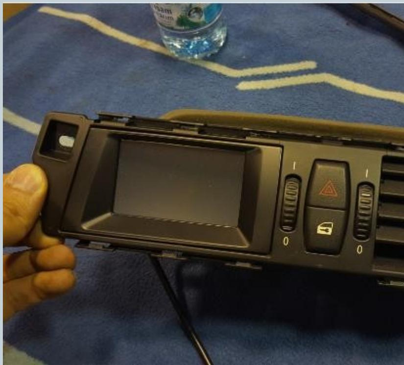
Replace the front part of the vent. **The lower side first.** Now the ventilation unit can be screwed to the interior trim again.
